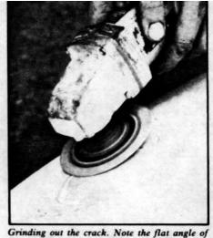
Grinding out the crack. Note the flat angle of attack of the grinderette. 80 grade paper is used.
